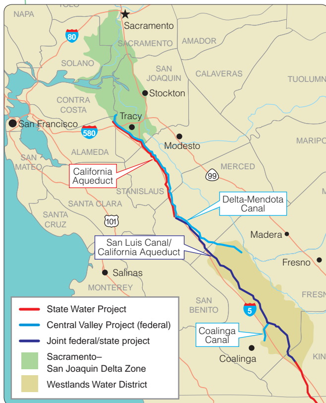
In California, water is pumped south with the help of state and federal canal systems.
